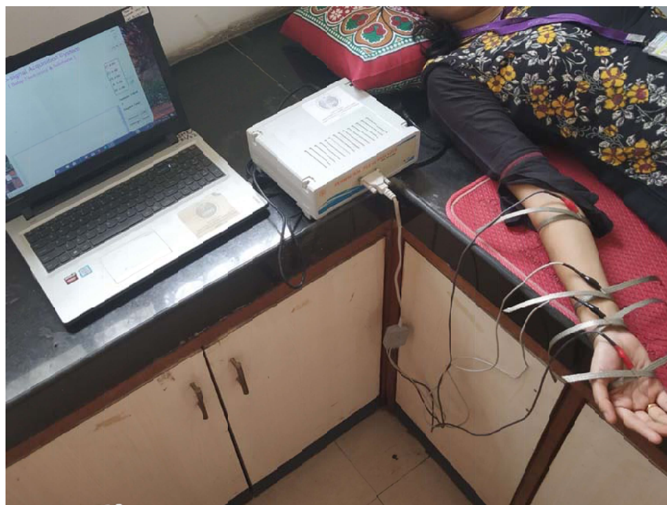
Fig. 1: Peripheral Pulse Analyzer instrument with electrodes attached to a control subject. Carrier electrodes C1 and C2 have red clips and sensing electrodes S1 and S2 have black clips seen on subject's hand.
